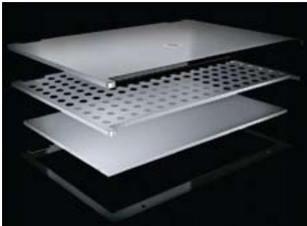
HP's DuraCase consists of an anodized aluminum top layer, thermally bonded to magnesium with a weight relief hole pattern, which protects the notebook's display while minimizing weight impact. © Photo courtesy of HP. Used with permission.
