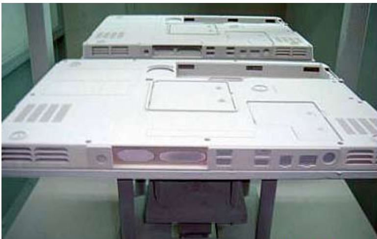
Primed magnesium alloy notebook cases on the paint line await their final high-tech finish coat.
