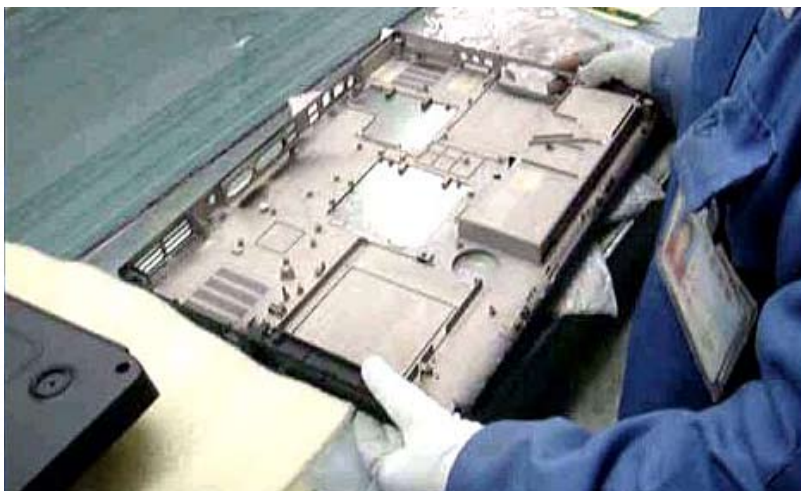
Componentry is well-protected as it is carefully installed into the magnesium notebook base on a subassembly line.
