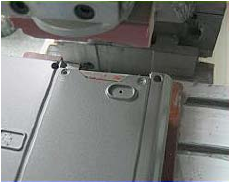
Magnesium alloy notebook base is positioned at a computer numerical control (cnc) center for secondary machining. Millions of units are manufactured to meet ever-increasing global demand.
