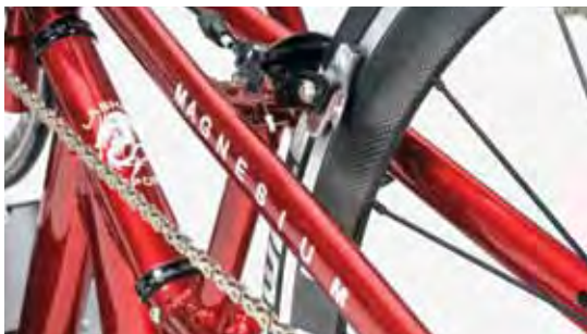
Its 100% magnesium parts make the Handcycle Elite light, fast and rigid, and efficiently dampen vibrations for a smoother ride. © Photo courtesy of Lasher Sport, LLC. Used with permission.
