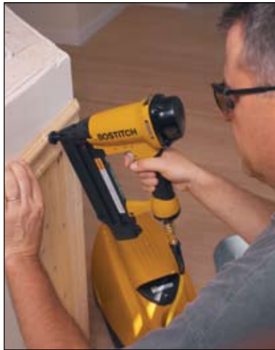
The lighter Bostitch magnesium oil-free brad nailer and narrow crown stapler have in-line magazines for better handling, balance and accuracy. Better ergonomics are possible when weight is reduced, resulting in less user fatigue issues during work shifts.
