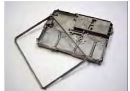
The ARMOR™ X10mg Rugged Tablet PC has a magnesium alloy chassis and sealed fanless design that delivers all-weather functionality for rugged outdoor computing. © Photo courtesy of DRS Tactical Systems, Inc. Used with permission.
