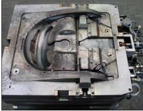
In phase one of the manufacturing process, this die-cast tool is used for the upper back portion of the chair.
