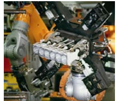
During production, specially designed aluminum insert on the toolset incorporates cylinder liners and coolant ducts for the magnesium-alloy engine.
