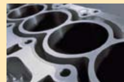
The R6 Composite Magnesium-Aluminum alloy engine is the mainstay of BMW's vehicle fleet.
