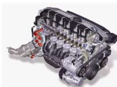
Magnesium alloy engine cross-section view shows Valvetronic® variable intake system, magnesium alloy crankcase, bedplate, and cylinder head covers.
