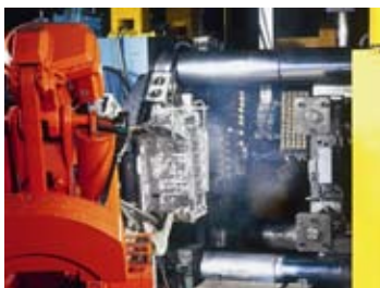
At the fully-automated Landshut plant, the magnesium alloy crankcase is removed from the world's largest die-casting machine
