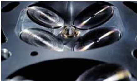
The cylinder head of the six-cylinder engine with BMW's technically advanced VALVETRONIC system.
